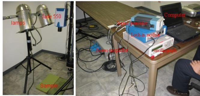
Fig 2 Cedip JADE MWIR 550 Lock-in thermography system
